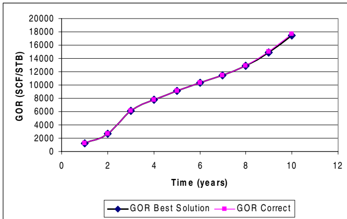
Fig. 12.-Gas oil ratio obtained using the best solution and the "correct" solution (Case Study No. 1)
